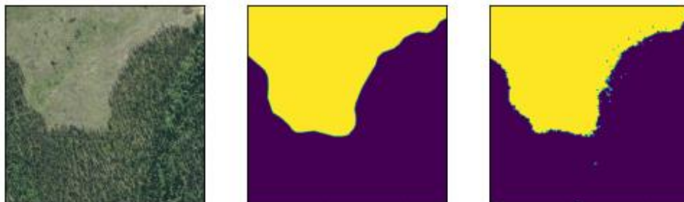
Figure 2: A sample tile (left), its labels (middle), and the predicted labels from the CNN model (right).
